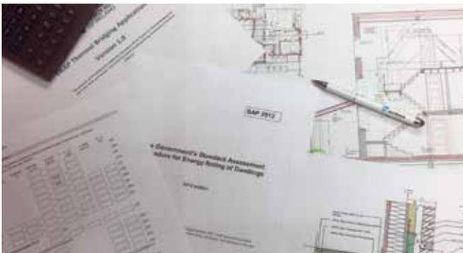
The heat loss through thermal bridges is accounted for in the SAP and SBEM, or in Ireland the DEAP and NEAP energy assessment calculation. This combines all the individual  $\psi$  values into a single  $\Psi$  value which is then added to the U value to give the total energy loss.
