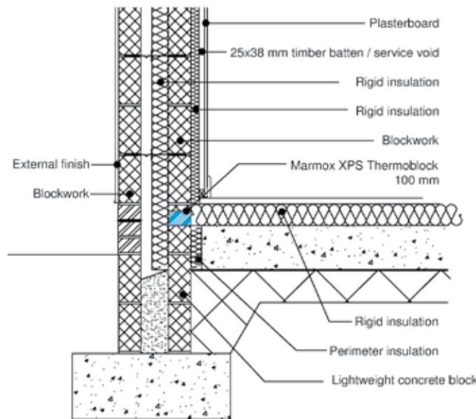
Using 100mm Marmox Thermoblock with 100mm wide aerated concrete/ AAC blocks.
