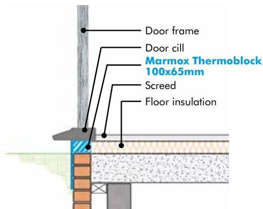
Marmox Thermoblock is suitable to use in the outer skin provided that its sides are protected from sunlight. The frame is mechanically fixed to the brickwork underneath the with a bolt or screw passing through the middle of the Thermoblock. Provided that the frame imposes its load evenly over the whole width of the Thermoblock, it may overhang the Thermoblock. Marmox sealant seals the Thermoblock to the frame.
