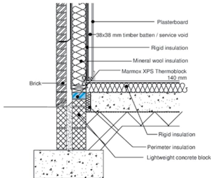
Using 140mm Marmox Thermoblock with 140mm wide timber frame.
