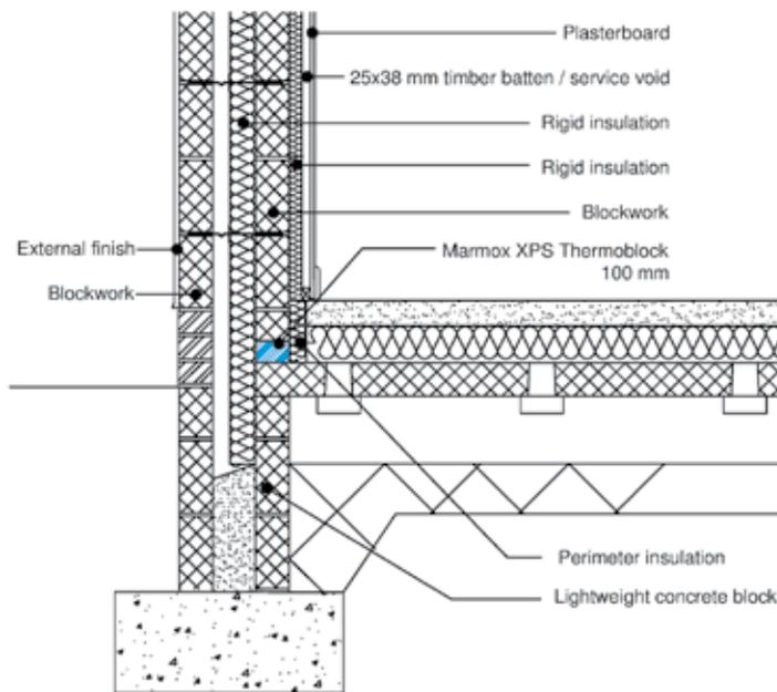
Using 100mm Marmox Thermoblock with 100mm wide aerated concrete/ AAC blocks.
