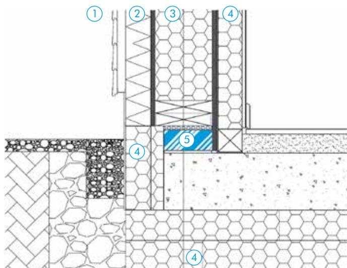
Marmox Thermoblocks are often incorporated into Passivhaus designs such as the example here. In addition to having a primary energy demand less than 120kWh/m<sup>2</sup>, very low U values, to achieve Passivhaus or zero carbon standards, the buildings need to be effectively thermal bridge free which means having a  $\psi$  value no more than 0.01W/mK. When used in the following design, Thermoblock resulted in making the junction a thermal bridge free.
