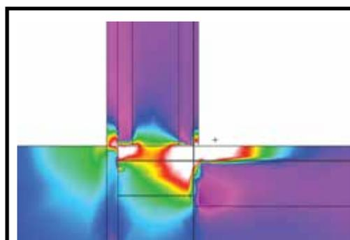
The  $\psi$  value of a typical ICF wall on a concrete slab is 0.15W/mK.
