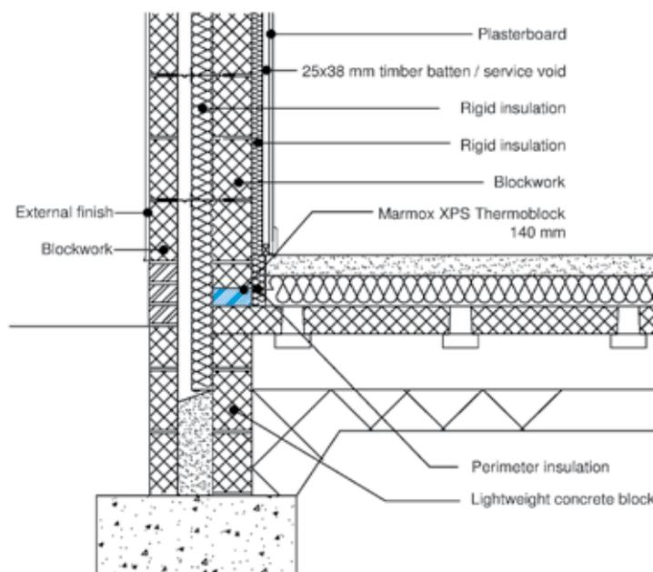
Using 140mm Marmox Thermoblock with 140mm wide aerated concrete/ AAC blocks.
